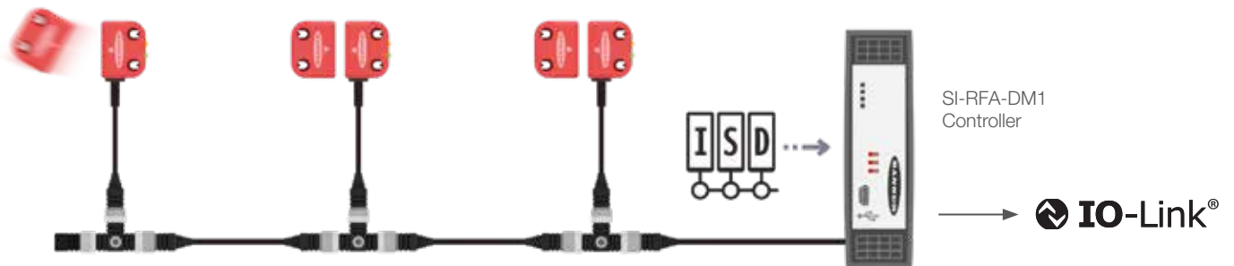
RFID SI-RF Switches – Cascade and ISD
